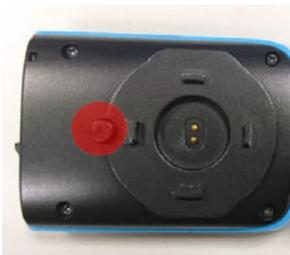
Step 2. Align the four grooves from the trigger module with MS652, also make sure arrows from both sides are close together. Please adjust the arrow alignment as shown in the photo below.
