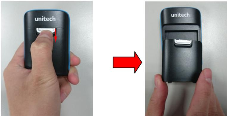
Step 2 : To install the battery, slide the battery and press down the latch to secure it until you hear the clicking sound.
